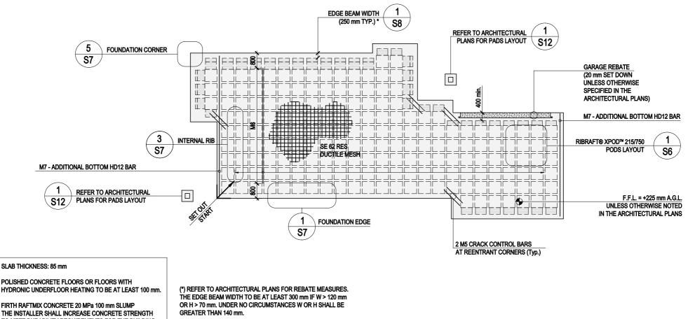
THE INSTALLER SHALL INCREASE CONCRETE STRENGTH TO MEET DURABILITY REQUIREMENTS FOR THE BUILDING SITE EXPOSURE ZONE AS REQUIRED (SEE SHEET 3)
